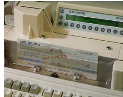
The documents in the hold-and-view station are perfectly visible when the operator must enter additional data from keyboard
