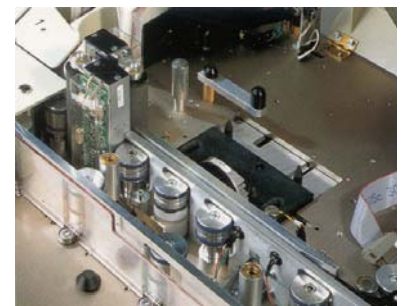
MICR or OCR encoder on RS85
